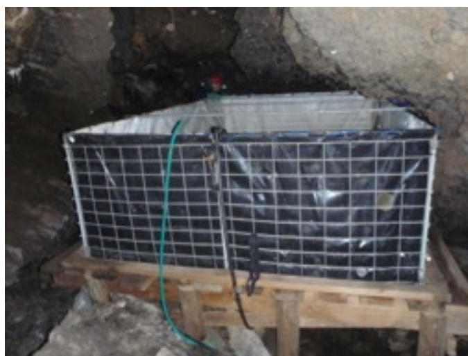
Plate 3: 16,000 litre holding tank in upper level of Short Creek passage.
